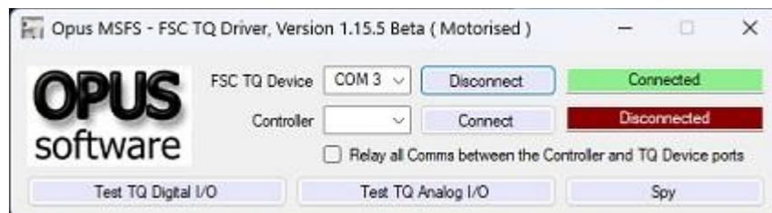
After connecting you should use the Test... dialogs to check and calibrate the interface with the Motorised TQ.
