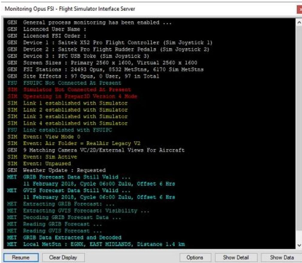
Spy indicates what joystick numbers have been mapped to each controller device. The button events within the Spy window will also indicate what physical device is currently mapped to the simulator's joystick number. The joystick order should match the controller order within the simulator's Controls Settings. If they don't then you can change the order via the **Remap Joystick Numbers** button in the Config dialog.
