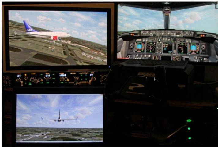
Live View Multi-Screen Networked Displays with CPFlight MCP and EFIS Panel drivers
